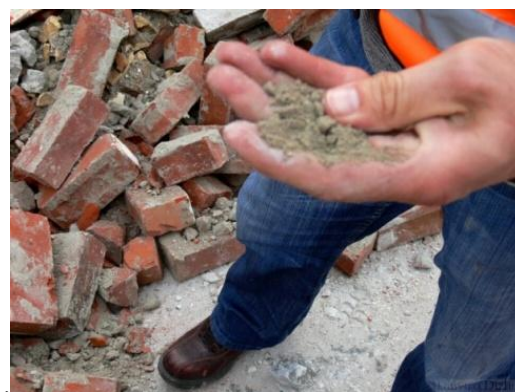
Figure 6: Example of weak mortar from damaged building.
